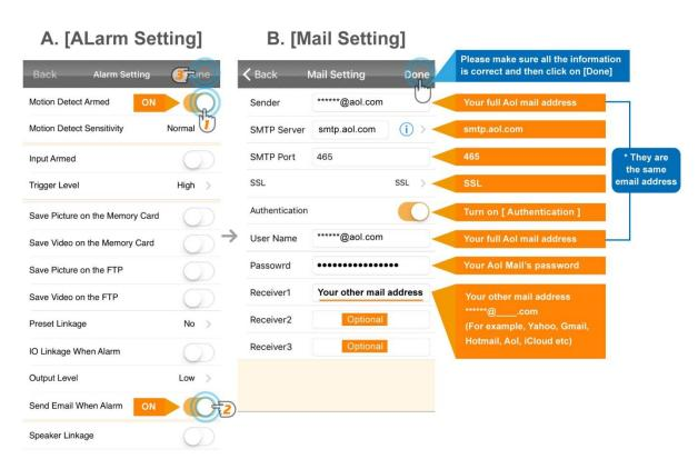
A. [Alarm Setting] → enable [Motion Detect Armed] and [Send mail When Alarm]. Tap [Done] (Tip: You can set Motion Detect Sensitivity to High, Normal, or Low. We suggest you to choose Normal)
